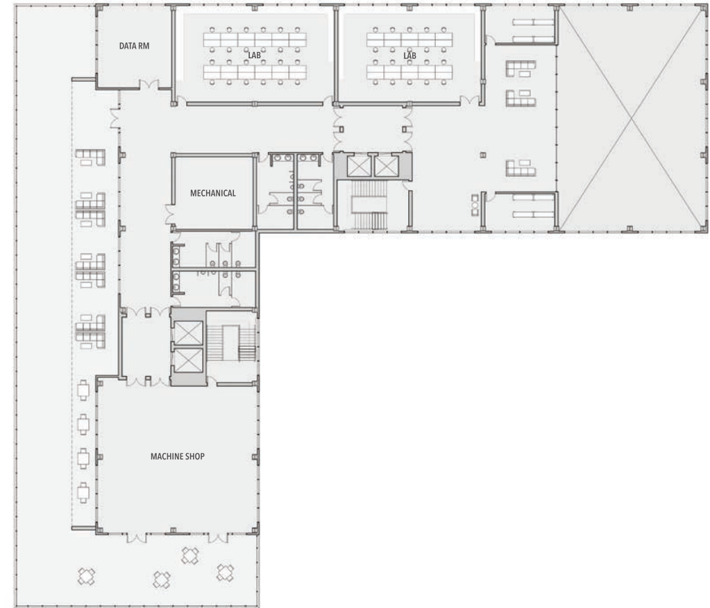
Fifth Floor Plan Contains two lab spaces and a machine shop, along with a large river-facing terrace.
