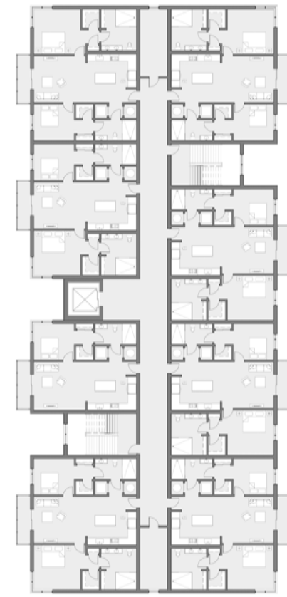
Apartment plans are organized to support density within the overall mixed-use system, with units positioned above retail and directly connected to the pedestrian spine that links the site's recreational and public spaces.
