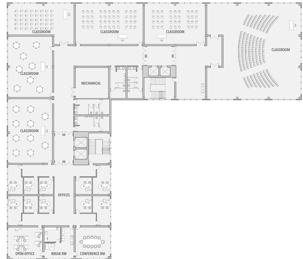
Third Floor Plan Classrooms and Offices arranged along a double-loaded corridor to ensure ample natural light.
